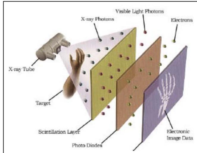
Figure 2: Flat Panel X-ray Detector<sup>1</sup>
