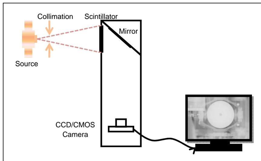
Figure 3: CCD/CMOS Camera System
